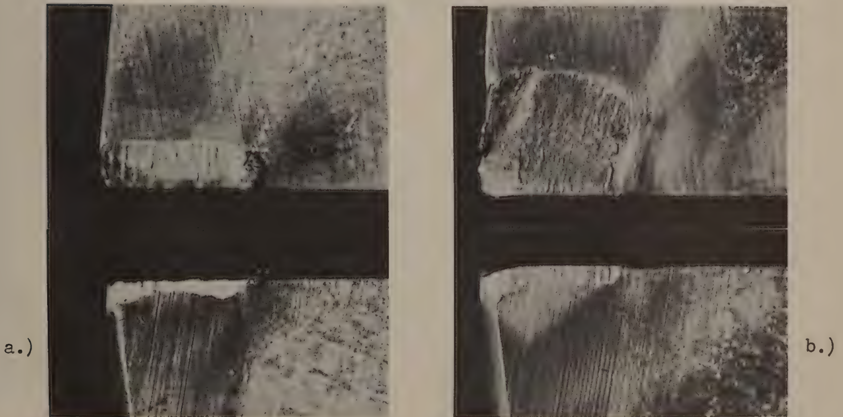
Fig. 43. Photographs of worn tools. Upper view shows chip face, lower view shows clearance face. Tool geometry: 0°, 0°, 5°, 5°, 5°, 0°, 0.015. a.) K-6 carbide tool used to cut titanium alloy at 345 fpm; feed, 0.0104 ipr; depth of cut 0.06 in., wear land, 0.014 in., fluid, none. b.) K-2S carbide tool used to cut 1045 steel at 485 fpm; feed, 0.0104 ipr; depth of cut, 0.060 in.; wear land, 0.0145 in.; cutting fluid, none.
